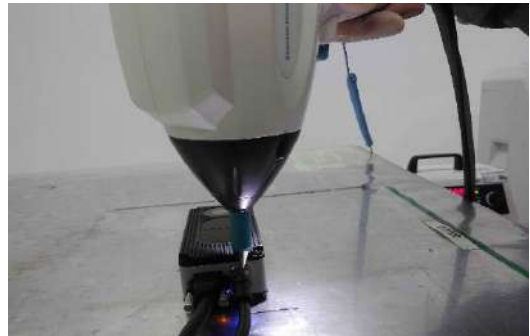
Contact discharge process
