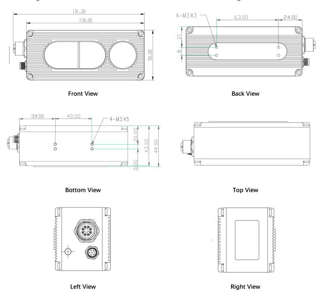
Fig. 3.2: ToF Camera Dimensions (Unit: mm)
