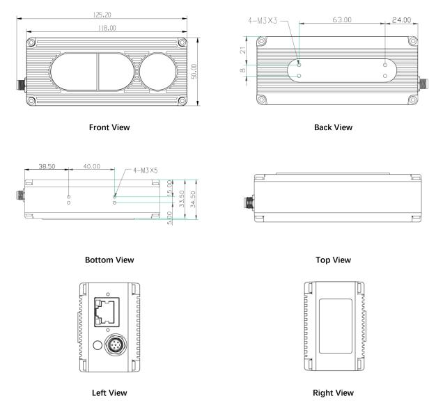
Fig. 3.1: ToF Camera Dimensions (Unit: mm)
